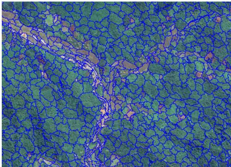
**Figure 3: Objects with multi-resolution segmentation (Scale parameter = 70, shape = 0.5, and compactness = 0.8)**
